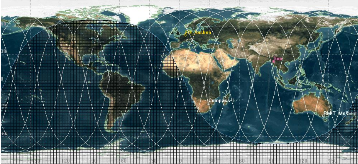
Figure 7: Ground track of Compass-1 for the reference orbit. Computed with STK's J4 propagator; (t=0 to 86400 s)
