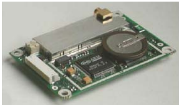
Figure 12: Phoenix (MG5001) receiver board
