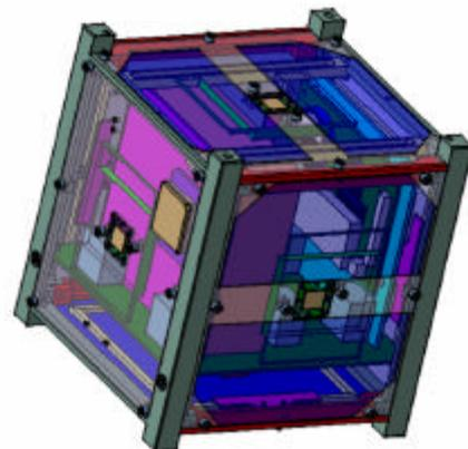
*Figure 1: Compass-1 CAD model*
